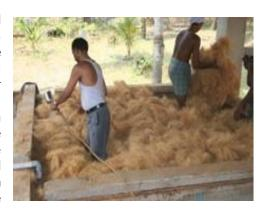
The bulk treatment of unwillowed fibre with oil in water emulsion was repeated on 1500 kg fibre on 02.02.06 using the same composition of 5g oil, 5g urea, 1.5g detergent and 125 ml water per kg fibre and kept in piled condition for 24 hours in RCC tank.
